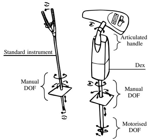
Figure 2: Standard and Dex instruments.
